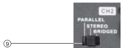
Mode Selector of 4-channel models
