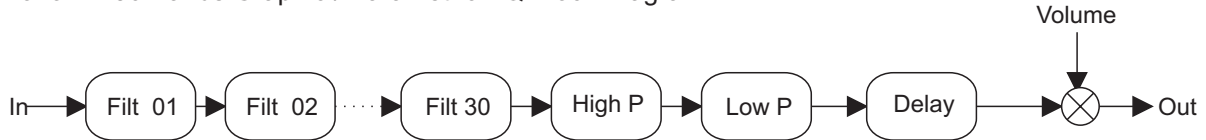
Mono 1 × 30 Bands Graphic / Parametric EQ Block Diagram
